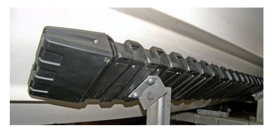
Position a new Snaptraxx bunk on the trailer drill a pilot hole through the bottom section and into the lumber to accept the lag bolts.
